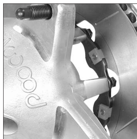
Wide 5 Racing Hub Assembly Showing T-Nut Placement with Rotor and Dynamic Mounting Plate. See Page 86.
