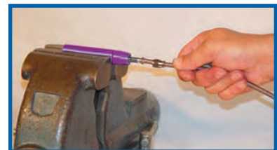
STEP FOUR Seat olive with a push.
