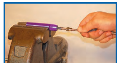
STEP TWO Flare braid using a twisting motion.
