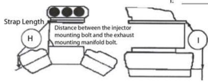
Distance between the back top of the blower and the top on the clutch can center bolt.
