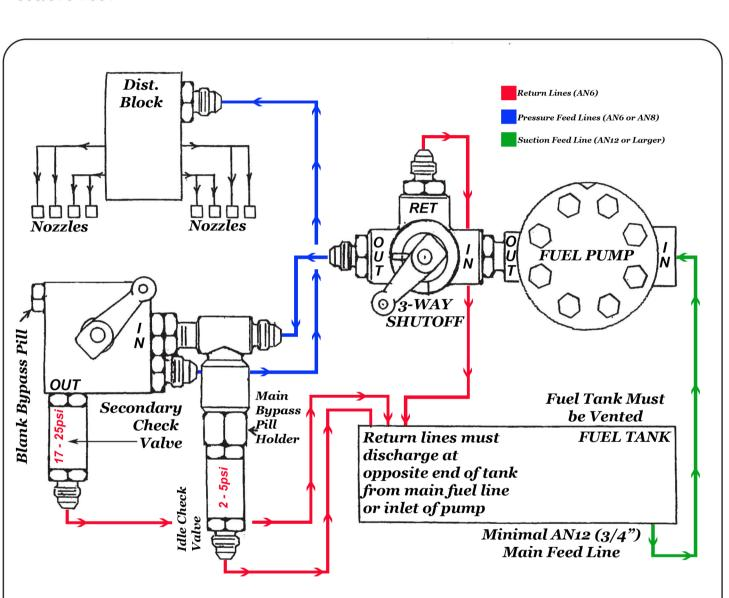
Most return lines can be looped back to the inlet of the fuel pump. This saves weight, cost and assembly time. For multiple return lines we recommend the use of a fuel log.
